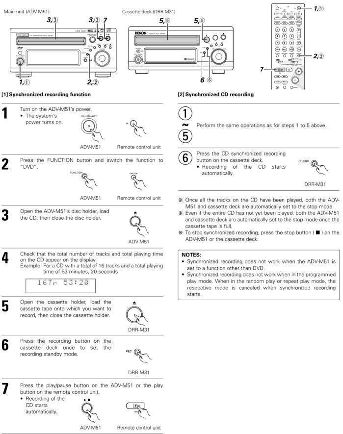
\* The recording standby mode is set once playback of the CD ends.
